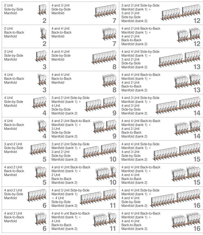
**NOTE**: When adding additional manifolds, field adjustment of the main piping may be necessary in order to properly connect the provided flex connectors to the water heaters.
