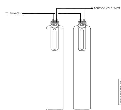
NUMBER OF PEAKFLOW C REQUIRED IS NOT EQUIVALENT TO NUMBER OF TANKLESS WATER HEATERS, PEAKFLOW C SIZING IS BASED ON FLOW RATE. SYSTEM DESIGN FLOW RATE IS 16 GPM PER TANK, 20 GPM PER TANK FOR INTERMITTENT USE ONLY. PEAKFLOW C CAN BE CASCADED UP TO 6 UNITS IN PARALLEL. PEAKFLOW IS NOT TO BE USED WITH TANK TYPE WATER HEATER OR TANK STORAGE. (REFER TO SIZING GUIDELINE FOR NAVIEN TANKLESS WATER HEATER ON NAVIENINC.COM)
