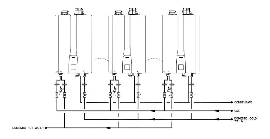
3 UNITS: 1-1/4" 4-5 UNITS: 1-1/2" 6-8 UNITS: 2" 9-14 UNITS: 2-1/2" 15-16 UNITS: 3" TANKLESS QUANTITY: RECOMMENDED PIPE SIZE 1 UNIT: 3/4" 2 UNITS: 1" SYMBOL LEGEND NPE-S2 SERIES TANKLESS WATER HEATER FULL-PORT VALVE UNION (3) NPE-S2 TANKLESS WATER HEATERS (INCLUDES NPE-A INTERNAL CIRCULATION MODE) 20 GOODYEAR IRVINE, CA 92618 .... CASCADE CABLE INCLUDES MODELS 150(NPE-S2 ONLY), 180, 210 AND 240 800-519-8794 S. STOEKE NPE-S2-3-I MAY 17, 2021 www.navieninc.com
