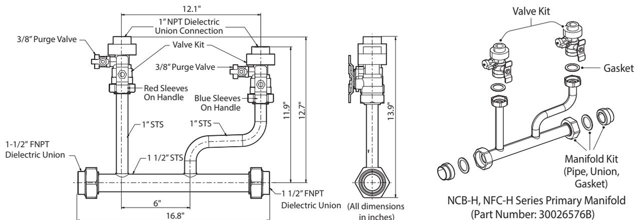
Check that a pipe, unions, gaskets, and valves are all included in the Manifold kit box and the Valve kit box. After installing the manifold and valve kits, ensure that the fittings, such as the unions and gaskets, are properly sealed with the pipe.
