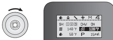
3. Press the Command dial (🌀) to select the DHW temperature (🔥). The highlighted section will flash.
