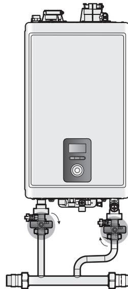
5. Remove the drain cap on the manifold system to drain the boiler.
