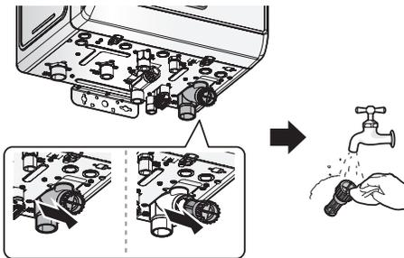
3. Reinsert and tighten the filter.
