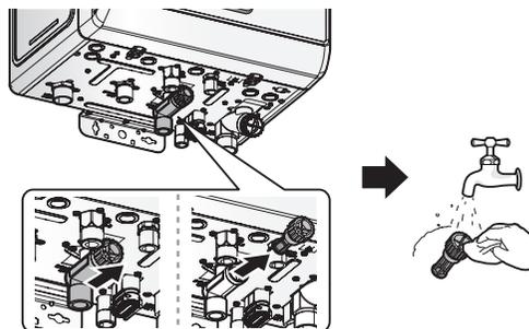
3. Reinsert and tighten the filter.
