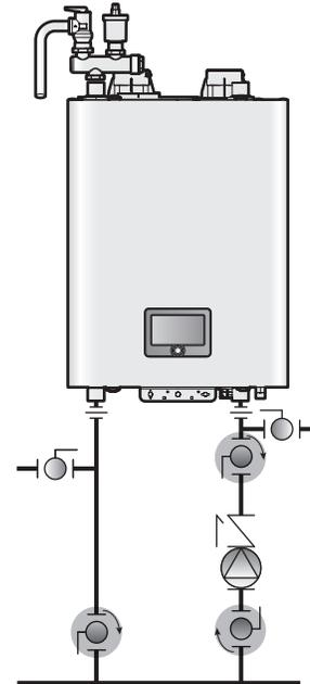
5. Remove the drain valve on the manifold system to drain the boiler.
