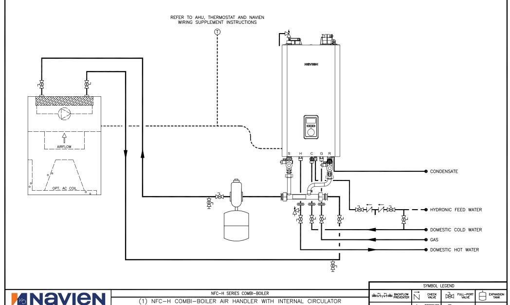
(1) NFC-H COMBI-BOILER AIR HANDLER WITH INTERNAL CIRCULATOR
