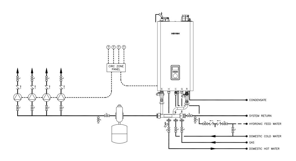
BACKFLOW PREVENTER FULL-PORT VALVE EXPANSION TANK NFC-H SERIES COMBI-BOILER MNavien THERMOSTAT (1) NFC-H COMBI-BOILER WITH MULTIPLE ZONE CIRCULATORS SHOWN WITH NAVIEN MANIFOLD KIT PART#30026576B AIR ELIMINATION MANIFOLD UNION 20 GOODYEAR IRVINE, CA 92618 INCLUDES MODELS NFC-250/175H, NFC-250/200H 800-519-8794 S. STOEKE NFC-H-1-4ZP-PLSS MARCH 7, 2023 www.navieninc.com
