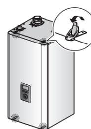
Unfasten the 4 latches (2 at the top and 2 at the bottom) to remove the front cover and gain access to the internal components.
