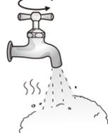
Open a hot water faucet. The boiler should turn on and the gas in the gas supply line will be purged.
