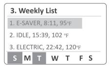
The set operation mode, time, and temperature will be displayed, while the selected days on the weekly schedule will be indicated at the bottom of the screen.
