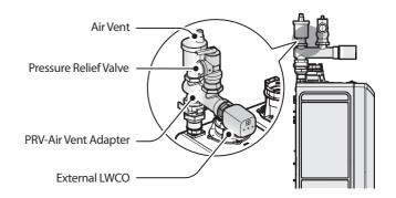
Figure 2. Adapter and Components Assembly (with LWCO)
