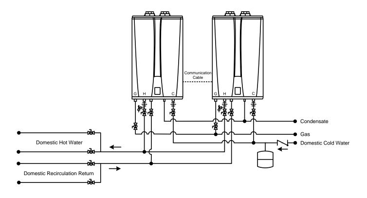
Recommended Pipe Size/Heater Count 1 Unit - 3/4" 2 Units - 1" 3 Units - 1-1/4" 4 to 5 Units - 1-1/2" 6 to 8 Units - 2" 9 to 14 Units - 2-1/2" 15 to 16 Units - 3"
