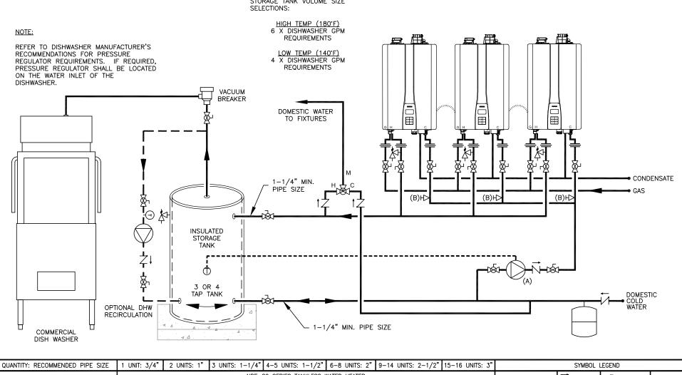
TANKLESS QUANTITY: RECOMMENDED PIPE SIZE NPE-S2 SERIES TANKLESS WATER HEATER FULL-PORT VALVE =AQUASTAT (3) NPE-S2 TANKLESS WATER HEATER DISHWASHER APPLICATION PRESSURI RELIEF VALVE 函 WITH STORAGE TO MEET FLOW/TEMP RISE REQUIREMENT ----- CONTROL WIRING CIRCULATOR 20 GOODYEAR IRVINE, CA 92618 INCLUDES MODELS 150, 180, 210 AND 240 800-519-8794 ₽ EXPANSION TANK S. STOEKE NPE-S2-3-DW-DHW-ST-1 SEPTEMBER 13, 2023 www.navieninc.com
