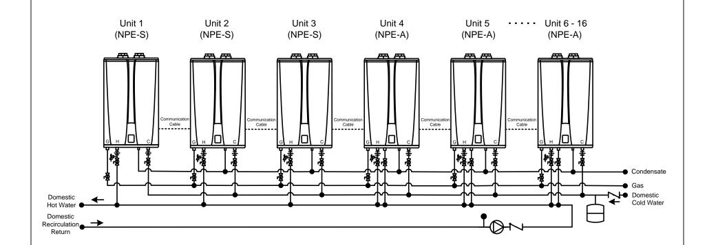
6 to 8 Units - 2" 9 to 14 Units - 2-1/2" Recommended Pipe Size/Heater Count 1 Unit - 3/4" 2 Units - 1" 3 Units - 1-1/4" 4 to 5 Units - 1-1/2" 15 to 16 Units - 3" NPE-A\S Series Tankless Water Heater
