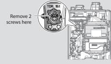
Figure 4. Access to Gas Orifice in Fan Assembly
