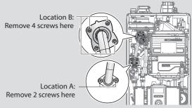
Figure 3. Detaching Gas Valve from Gas Inlet Pipe and Fan Motor Assembly
