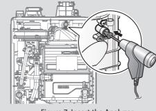
Figure 7. Insert the Analyzer
