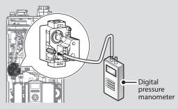
Figure 9. Connect Digital Pressure Monometer
