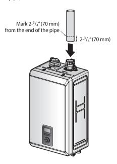
2. Insert the pipe into the vent collar to start the vent run. Make sure to completely slide the vent into the collar until the end makes contact with the bottom of the socket.
