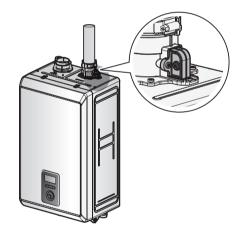
As shown, the VID is a device connected to the vent collar which is intended to detect whether the vent pipe has been inserted to a sufficient depth into the collar during its initial installation.
