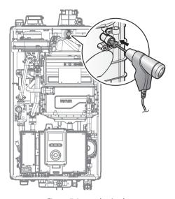
Figure 7. Insert the Analyzer
