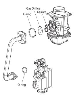
Figure 5. Exploded View of Gas Pipe Assembly
