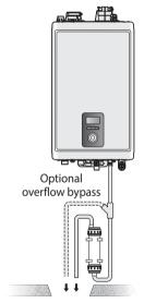
Figure 2. Vertical installation
