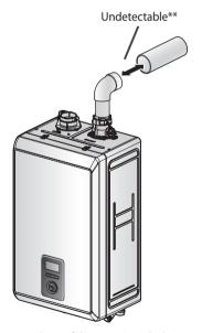
\*\*VID can not detect if the vent pipe is leaking or disconnected at any point between the boiler and the exterior vent location or if the vent is blocked for any reason.
