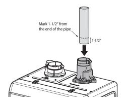
Insert the vent pipe into the vent collar to start the vent run. Make sure to completely slide the vent into the collar until the end makes contact with the bottom of the socket.
