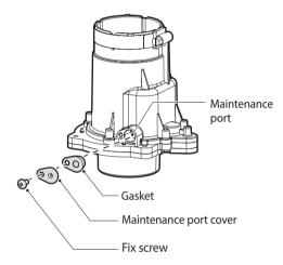
Through the maintenance port, check the operating condition of the damper plate inside the Common Vent Collar Kit.
