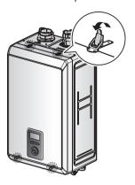
Loosen the screws indicated in the figure below and connect a manometer to the pressure port.
