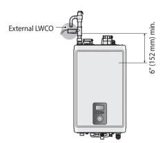
Figure 1. External LWCO (without Navien Manifold System)
