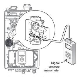
Figure 9. Connect Digital Pressure Monometer
