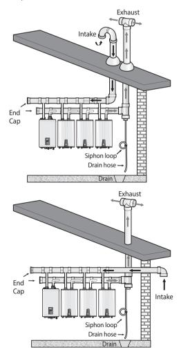
To install a condensate drain to the cascade system:
