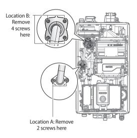
Figure 3. Detaching Gas Valve from Gas Inlet Pipe and Fan Motor Assembly
