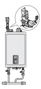
Figure 2. External LWCO (with Navien Manifold System)
