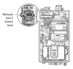
Figure 4. Access to Gas Orifice in Fan Assembly
