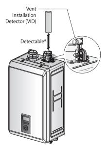
\*If inserted  $2^{-3}/_4$ " (70 mm), then VID should detect vent pipe.
