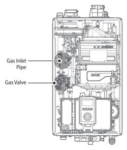
Figure 2. NCB-H Series Internal Components
