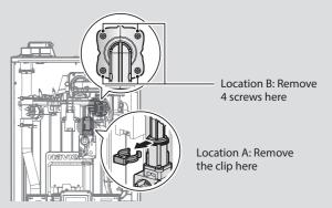
Figure 3. Detaching the Gas Valve Outlet Adapter from the Gas Valve and Fan Motor Assembly
