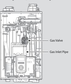
Figure 2. NFB-H Series Internal Components
