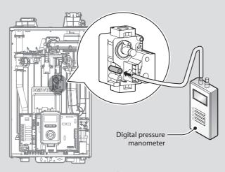
Figure 8. Connect Digital Pressure Manometer
