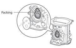
9. Replace the gas valve outlet adapter to its original position and use all screws to secure all connections.
