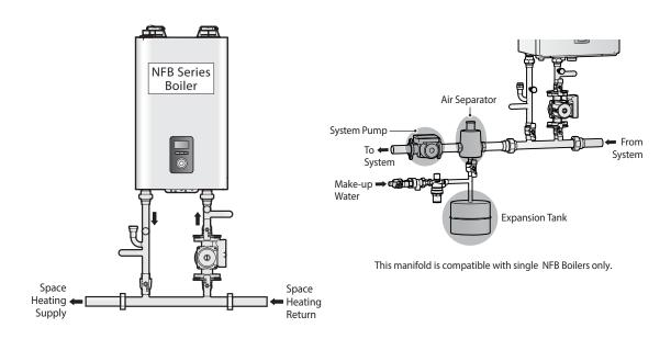
NFB-175/200 Series Manifold Piping Setup with Accessories
