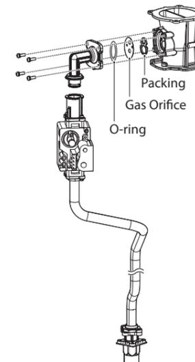
Figure 5. Exploded View of Gas Pipe Assembly
