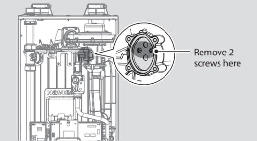
Figure 4. Access to Gas Orifice in Fan Assembly
