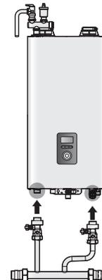
FIGURE 1. Supply and Return Fittings on the Navien NFC Boiler with Connection Sizes
