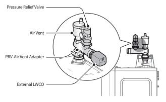
Figure 3. Adapter and Components Assembly (with LWCO)
