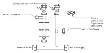
Figure 3. Available Ports on the NHB-H Series Primary Manifold
