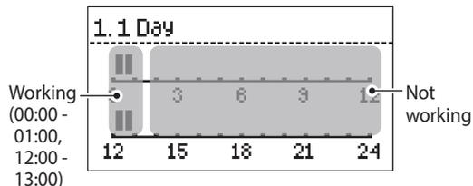
Press the Up button (▲) or the Down button (▼) to choose the scheduled time. You can choose the time in 30 minutes intervals. To finalize the weekly schedule settings, press and hold the OK button (OK) for more than 2 seconds.
