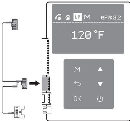
**Note** If a longer connection is required, the two can be connected and extended.
