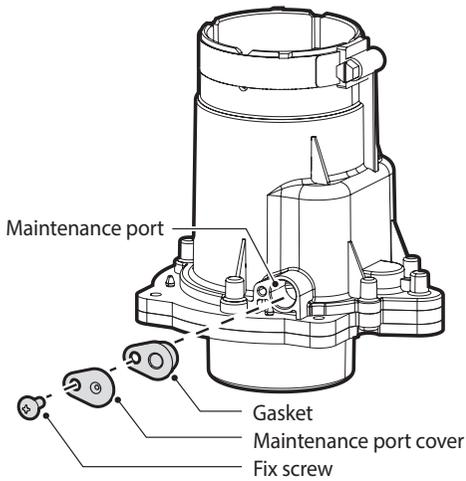
Refer to "6.8 Maintenance" for detailed inspection procedures of the Navien Common Vent Collar Kit (Back-draft Damper).
