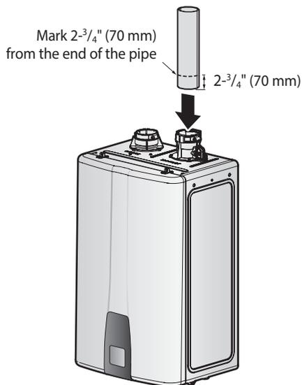
2. Insert the pipe into the vent collar to start the vent run. Make sure to completely slide the vent into the collar until the end makes contact with the bottom of the socket.
