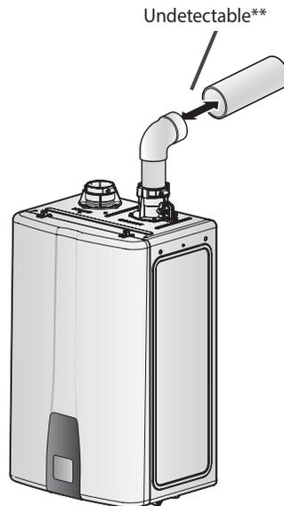
\*\*VID can not detect if the vent pipe is leaking or disconnected at any point between the water heater and the exterior vent location or if the vent is blocked for any reason.
