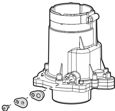
**Note** If condensate comes out the port when opened, check for proper drainage or any blockage.
