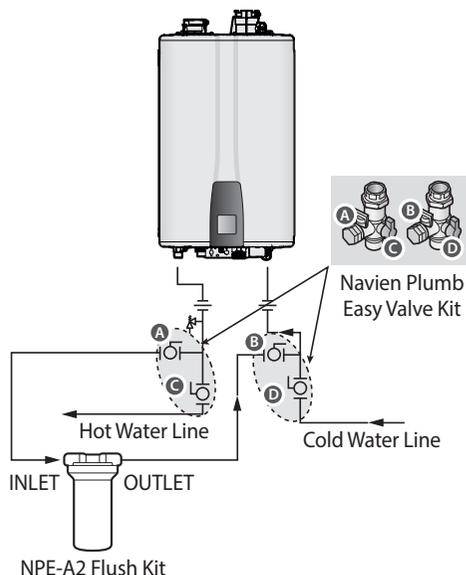
To flush the Heat Exchanger: NPE-S2 Model
