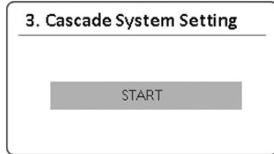
3. Press and hold the OK button (OK) for 3 seconds on the sub unit. Then, the **ID 1. Allocated!** message will appear on the sub unit's front panel display. When the water heater is set to a sub unit, the **S** icon will appear on the display.
