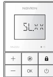
3. When the ID is assigned, the ID appears and flashes on the LCD display for 2 seconds.
