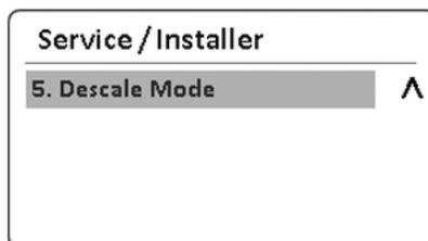
2. Press the Up button (▲) or the Down button (▼) to switch between the descaling time. Press the OK button (OK) to select a parameter or to run the descale mode.
