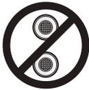
Do not vertically stack concentric terminations on sidewalls. The circulation of exhaust gases will cause improper operation of the water heater.
