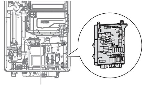
4. Connect the external pump wiring connector to the connector socket on the PCB (TB1).
