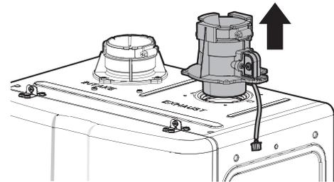
3. Connect the Common Vent Collar Kit to the exhaust duct of the water heater unit.
