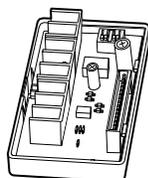
The NPE-A2/S2 series water heaters have a built-in Navien HotButton controller (the push button, wall plate, and temperature sensor have to be purchased separately). It adds signal input functions to the NPE-A2/S2 series water heaters for more efficient DHW hot water recirculation functionality.
