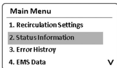
2. Press the Up button (▲) or the Down button (▼) to switch between the information items. Press the OK button (OK) to select an item and view its information.
