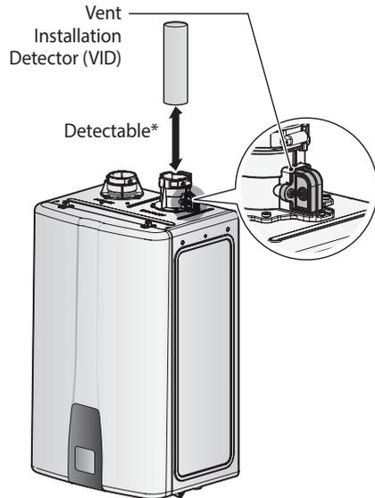
\*If inserted  $2\text{-}\frac{3}{4}\text{'}$  (70 mm), then VID should detect vent pipe.
