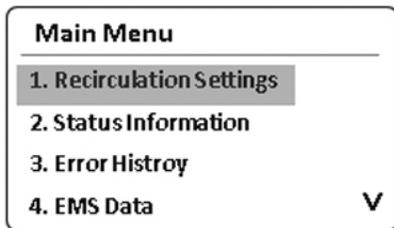
2. Press the Up button (▲) or the Down button (▼) to switch between the information items and press the OK button (OK) to select an item.
