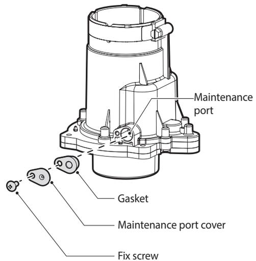
2. Through the maintenance port, check the operating condition of the damper plate inside the Common Vent Collar Kit.
