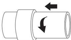
3. Hold the pipe and pipe fitting together for about 15 seconds until the cement sets.
