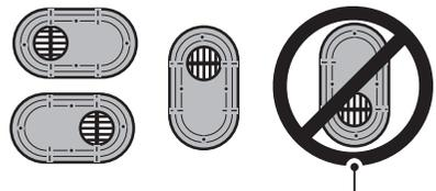
NEVER install in this orientation with the exhaust located nearest to the ground.
