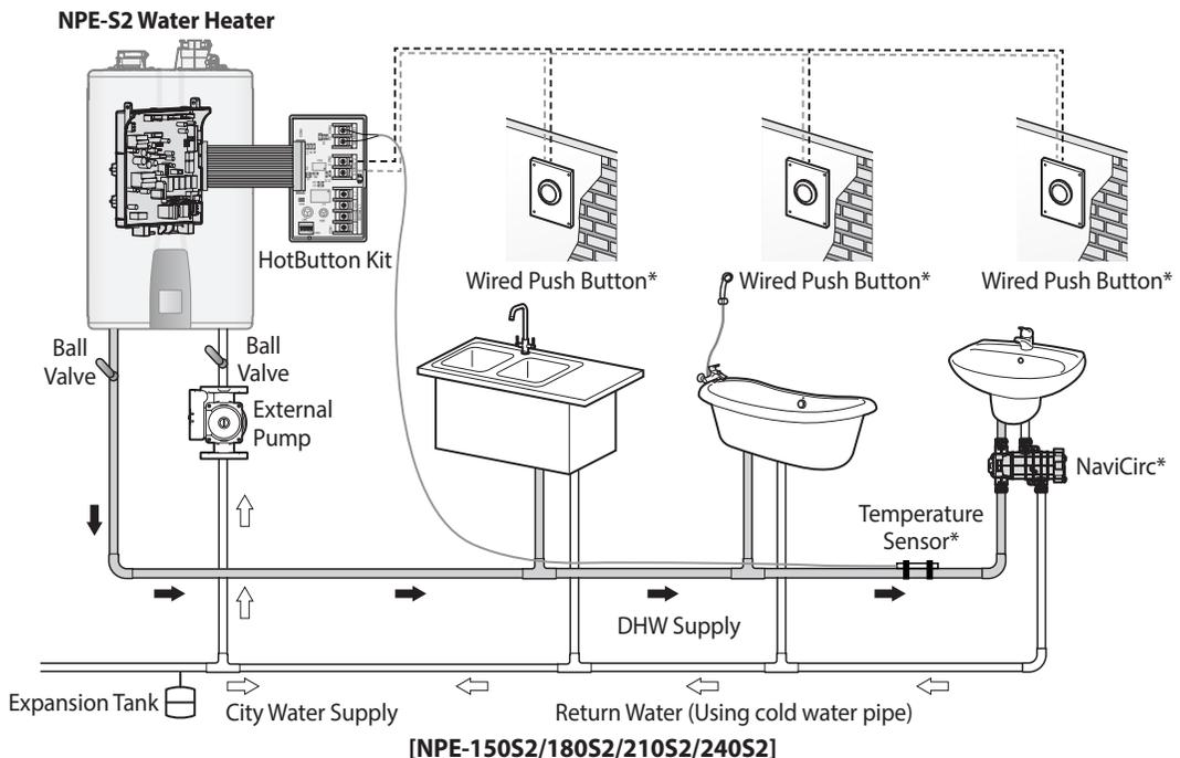
\*The NaviCirc recirculation valve, the push buttons, and the temperature sensor are not included with the water heater but are available for purchase.
