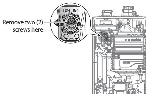
Figure 4. Access to Gas Orifice in Fan Assembly
