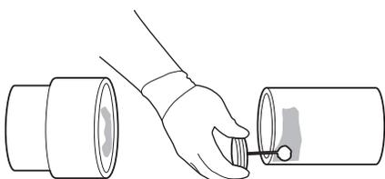
2. Align the pipe with the pipe fitting and twist the pipe a quarter turn as you insert it into the fitting. Twisting the pipe spreads the solvent cement evenly to ensure a solid joint.
