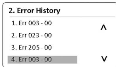
2. Press the Up button (▲) or the Down button (▼) to switch between the list of errors. Press the OK Button (OK) to select an error to view detailed information.
