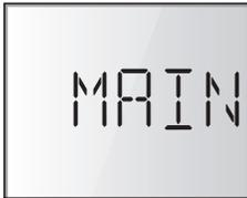
The remote controller that does not display "MAIN" is already operating as the main controller, you don't have to set its operation mode.
