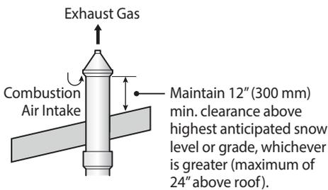
**Note** For cascade applications, the required horizontal clearance between terminations is 12" for both sidewall and vertical venting installations.
