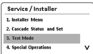
2. Press the Up button (▲) or the Down button (▼) to switch between the test procedures. Press the OK button (OK) to select a parameter or to run a test procedure.
