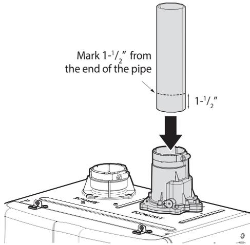
2. Insert the vent pipe into the vent collar to start the vent run. Make sure to completely slide the vent into the collar until the end makes contact with the bottom of the socket.
