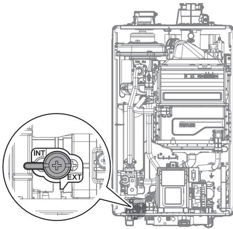
3. Press the Menu button (M) to access the Main menu and select **1. Recirculation Setting** > **3. Internal Recirculation** by pressing the OK button (OK).
