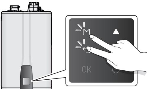
2. Select **2. Cascade Status and Set** > **3. Cascade System Setting** by pressing the OK button (OK). Then the **START** button will appear on the main water heater's front panel display. Press the OK button (OK) to start the cascade system setting.
