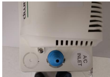
Figure 2: AC (Air Conditioning) inlet located beside check valve on top of the pump
